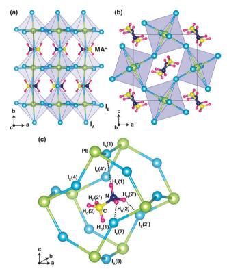
Fig. 1 (a) Optimized crystal structure of o-MAPbl $_3$ , viewed in the a-b and, (b) a-c planes. Pbl $_6$  octahedra are highlighted in purple. (c) Local cage structure of o-MAPbl $_3$  is characterized by hydrogen-bonding between the three H atoms in the NH $_3$  group and one axial I [I $_4$ (1)] atom and two equatorial I [I $_6$ (2) and I $_6$ (2')] atoms. Hydrogen-bonding interactions are indicated by dotted lines.
