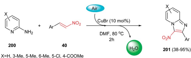
Scheme 68 Cu-catalyzed synthesis of imidazo[1,2- a ]pyridines.
