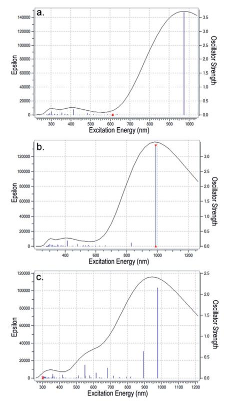
Fig. 7 The UV-vis spectra for (a) PEDOT $^{2+}$  (without PSS $^{2-}$  counterion); (b) PEDOT $^{2+}$  slightly bent to interact with the dianion; and (c) PEDOT $^{4+}$ with more bending when it interacts with the tetracation.
