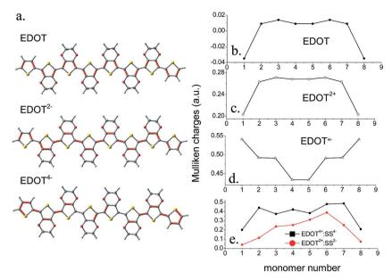
Fig. 5 (a) Nature of bond alternation in EDOT, EDOT $^{2+}$  and EDOT $^{4+}$ . The red bonds are aromatic double bonds (1.38–1.39 Å for C=C and 1.70 Å for C=S). (b) Mulliken charges for EDOT. (c) Mulliken charges for EDOT $^{2+}$ . (d) Mulliken charges for EDOT $^{4+}$ . (e) Mulliken charges for EDOT $^{2+}$  and EDOT $^{4+}$ -SS $^{2-}$  and EDOT $^{4+}$ -SS $^{4-}$ .
