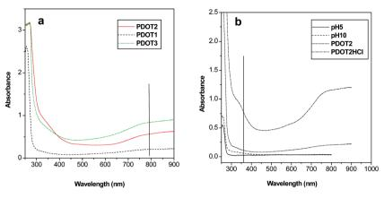
Fig. 3 UV-vis absorption spectra of PEDOT-PSS solutions at (a) different concentrations and at (b) different pH values.
