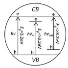
Fig. 7 Simplified relative energy bad positions and band widths for pure  $(h\nu)$  metal doped  $(h\nu_{\rm m})$  and non-metal doped  $(h\nu_{\rm nm})$  TiO<sub>2</sub> anatase.197
