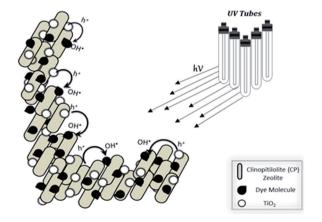
Fig. 8 Synergistic effect of TiO<sub>2</sub> and clinopitilolite catalyst on dye degradation by producing OH free radicals.318
