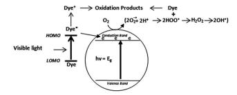
Fig. 3 Pictorial representation of direct dye degradation process.
