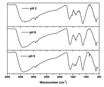
Fig. 7 FTIR spectra of sludge produced at various solution pHs.
