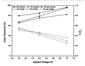
Fig. 2 Effect of applied voltage on COD and color removal efficiencies of the EF, PC and PC-pH processes at pH 3, ferric ion dosage of 10 mg  $L^{-1}$ , electrode area of 25 cm<sup>2</sup>.
