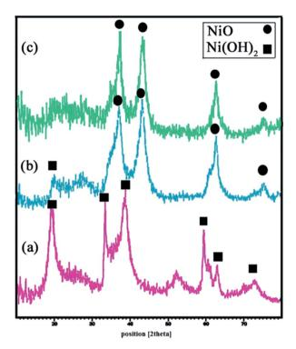
Fig. 3 XRD patterns of (a)  $\beta$ -Ni(OH)<sub>2</sub>, (b and c) 6 hours calcined  $\beta$ -Ni(OH)<sub>2</sub> at 700 °C and 750 °C, respectively.
