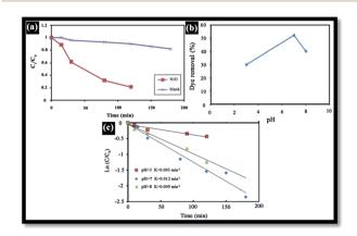
Fig. 8 (a) Variation in RB concentration with time (NiO dose (W) = 1 g L  $^{-1}$ , [RB] = 10 mg L  $^{-1}$ , pH = 7), (b) pH effect on the removal of RB dye (NiO dose (W) = 1 g L  $^{-1}$ , [RB] = 10 mg L  $^{-1}$ , T = 20  $^{\circ}$ C, t = 12 h), (c) effect of the initial pH on the photocatalytic degradation of RB dye (NiO dose (W) = 1 g L  $^{-1}$ , [RB] = 10 mg L  $^{-1}$ ).
