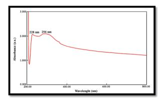
Fig. 5 UV-vis spectrum of the NiO nanoparticles.
