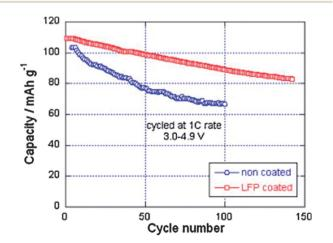
Fig. 17 Cyclability of the Li//LMN and Li//LFP-coated LMN cells at 1 C between 3.0 and 4.9 V vs. Li $^+$ /Li $^0$ . Reproduced with permission.
