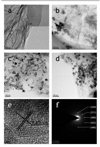
**Fig. 1** TEM images of RGO (a), RGO–Fe $_3$ O $_4$ -1 composite (b), RGO–Fe $_3$ O $_4$ -2 composite (c), RGO–Fe $_3$ O $_4$ -3 composite (d); HRTEM image (e) and SAED pattern (f) of RGO–Fe $_3$ O $_4$ -2 composite.
