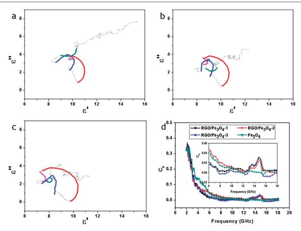
Fig. 9  $\varepsilon'$ - $\varepsilon''$  curves of RGO-Fe<sub>3</sub>O<sub>4</sub>-1 composite (a), RGO-Fe<sub>3</sub>O<sub>4</sub>-2 composite (b) and RGO-Fe<sub>3</sub>O<sub>4</sub>-3 composite (c);  $C_0$ -f curves of Fe<sub>3</sub>O<sub>4</sub> NPs and RGO-Fe<sub>3</sub>O<sub>4</sub> composites (d), inset is the expansion of the curves.
