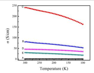
**Fig. 3** Temperature dependence of the electrical conductivity of the prepared samples: (A) pure PEDOT:PSS nanofilm, (B) SWCNTs/PEDOT:PSS layered nanostructure, (C) SWCNTs/PEDOT:PSS (doped with DMSO) layered nanostructure, (D) SWCNTs/PSS layered nanostructure, (E) SWCNTs/PVA layered nanostructure.
