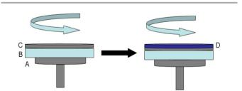
**Fig. 1** Schematic illustrations of the process in preparation of layered nanostructure: (A) metal tray, (B) glass substrate, (C) SWCNTs nanofilm, (D) PEDOT:PSS nanofilm.
