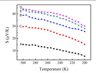
**Fig. 6** Temperature dependence of the Seebeck coefficient of the prepared samples: (A) pure PEDOT:PSS nanofilm, (B) SWCNTs/PEDOT:PSS layered nanostructure, (C) SWCNTs/PEDOT:PSS (doped with DMSO) layered nanostructure, (D) SWCNTs/PSS layered nanostructure, (E) SWCNTs/PVA layered nanostructure.
