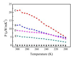
**Fig. 7** Temperature dependence of the power factor of prepared samples: (A) pure PEDOT:PSS nanofilm, (B) SWCNTs/PEDOT:PSS layered nanostructure, (C) SWCNTs/PEDOT:PSS (doped with DMSO) layered nanostructure, (D) SWCNTs/PSS layered nanostructure, (E) SWCNTs/PVA layered nanostructure.
