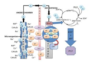
**Fig. 6** A schematic of the sMFC displaying the process occurring at the anode and cathode during the power generation. The anode and cathode electrode were carbon cloth and MnO<sub>2</sub>-NTs were supported on the different forms of carbon, respectively. Nafion 117 was used as the cation exchange member in the current sMFC test.
