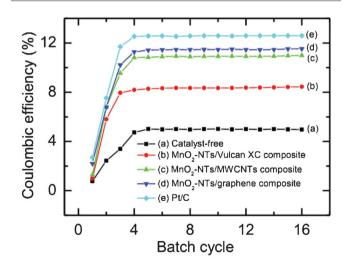
**Fig. 7** Coulombic efficiency (%) of sMFC as a function of batch cycle with (a) catalyst-free, (b) MnO<sub>2</sub>-NTs/Vulcan XC, (c) MnO<sub>2</sub>-NTs/MWCNTs, (d) MnO<sub>2</sub>-NTs/graphene, and (e) Pt/C composite cathodes. Each batch cycle was 36 h ( $\pm 2$  h).
