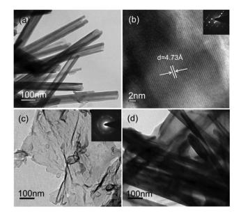
Fig. 1 TEM images of (a) hydrothermally synthesized MnO<sub>2</sub>-NTs, (b) lattice from the wall of MnO<sub>2</sub>-NTs, (c) graphene and (d) MnO<sub>2</sub>-NTs/graphene composite. Insets of (b) and (c) show the SAED patterns.
