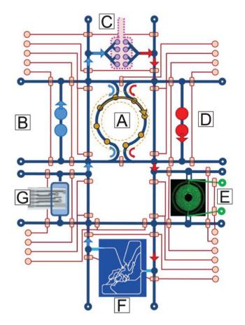
Fig. 3 A concept drawing of a four-organ μHu (Homo chippiens). A) An on-chip peristaltic ventricular assist, B) Right heart, C) Lung, D) Left heart, E) Liver (courtesy of Kapil Pant), F) Peripheral circulation 118 (courtesy of Kapil Pant), G) Microchemical analyzer of metabolic activity. 119 The system would operate on a single microfluidic chip, with on-chip pneumatic valves controlling system functions and connections.
