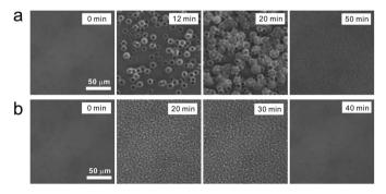
Fig. 14 (a) NG-type pattern evolution during LLT at  $T=180~{\rm K}$  for c=0.165. (b) SD-type pattern evolution at T = 173 K for c = 0.165. In both cases, the initial state is liquid I and the final state is liquid II. The patterns were observed with phase contrast microscopy. White bars correspond to 50 μm.
