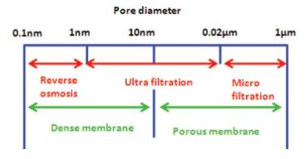
Fig. 2 Filtration spectrum; micro-, ultra-filtration and reverse osmosis.
