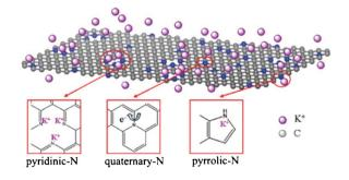
**Fig. 7** Scheme of the electrochemical reaction process of NGS materials in 6 M KOH electrolyte.
