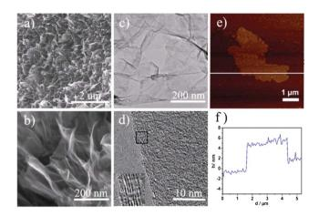
**Fig. 1** a, b) SEM, c) TEM and d) HR-TEM images of the NGS-1(mass ratio of urea/GO is 300 : 1, 180 °C, 12 h); e) Representative AFM image and f) corresponding thickness analysis taken around the white line in e) reveal a thickness of 4–4.5 nm for NGS-1.
