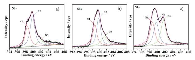
Fig. 4 XPS N1s spectrum of the NGS prepared with different hydrothermal reaction times: a) NGS-9 (4 h), b) NGS-10 (8 h) and c) NGS-11 (16 h).
