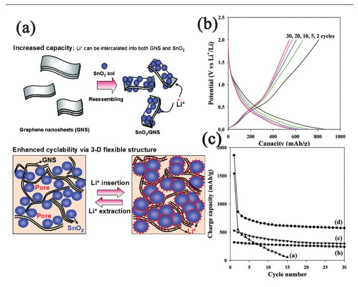
Fig. 13 (a) Schematic illustration for the synthesis and structure change of GN–SnO<sub>2</sub> nanocomposite during Li<sup>+</sup> insertion and extraction. (b) Charge–discharge profile for GN–SnO<sub>2</sub> nanocomposite. (c) Cyclic performances for (a) bare SnO<sub>2</sub> NPs, (b) graphite, (c) GN, and (d) GN–SnO<sub>2</sub> nanocomposite. Reprinted with permission from ref. 450. Copyright 2009, American Chemical Society.
