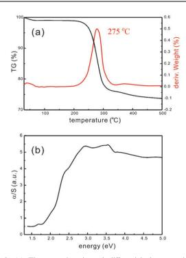
Fig. 3 (a) Thermogravimetric and differential thermogravimetric curves of H-Re/Te/Mn under nitrogen flow (heating rate 10 °C min<sup>-1</sup>). (b) Solid state UV/Vis spectrum of H-Re/Te/Mn. Absorption data were calculated from the reflectance data using the Kubelka-Munk function;  $\alpha/S = (1 - R)^2/2R$ , where R is the reflectance at a given wavenumber,  $\alpha$  is the absorption coefficient, and S is the scattering coefficient. The band gap energy is 1.92 eV.
