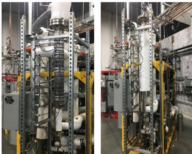
**Figure 2.** Pilot-scale reactor with (left) and without (right) insulation, where band heaters are visible and wrapped around the reactor. The full piping and instrumentation diagram is available in Figure S6 of the Supporting Information.
