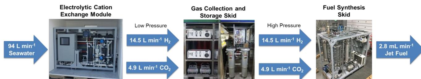
**Figure 13.** US Naval Research Laboratory modular seawater-to-fuel system consisting of an electrolytic cation exchange module (E-CEM), gas collection and storage skid and fuel synthesis skid. The pilot-scale system can produce up to four liters of jet fuel per day ( $2.8 \text{ mL min}^{-1}$ ).
