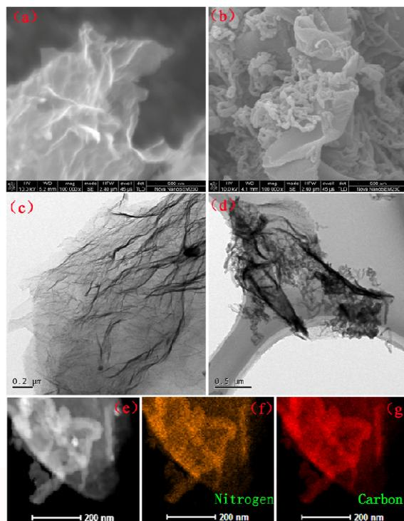
Fig. 2 SEM images of (a) graphene (RGO), (b) graphene/nitrogen-doped porous carbon nanofiber (RGO/NPC). TEM image of (c) RGO, (d) RGO/NPC. (e) Annular dark-field TEM image, and corresponding (f) nitrogen and (g) carbon elemental mapping of RGO/NPC .
