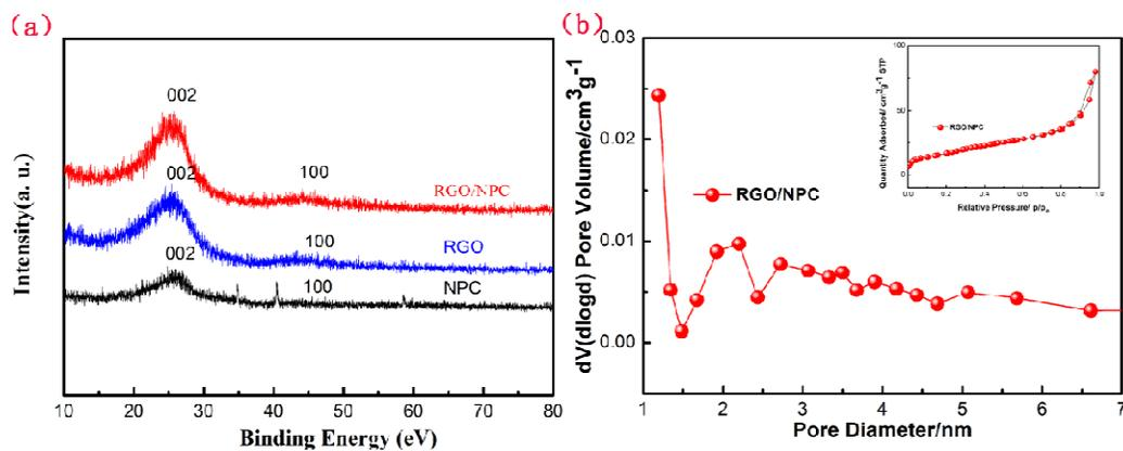
Fig. 3(a) XRD pattern of the RGO, NPC and RGO/NPC. (b) The pore size distribution of RGO/NPC, the inset picture displays N<sub>2</sub> adsorption-desorption isotherms.
