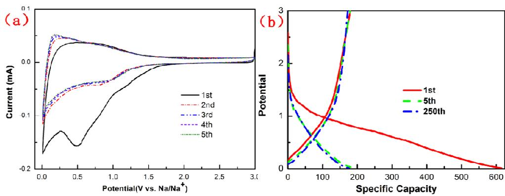
Fig. 5(a) Typical CV curves of the RGO/NPC electrode at a potential sweep rate of  $0.2 \text{ mV s}^{-1}$  and (b) The 1st, 5th and 200th charge-discharge profiles of the RGO/NPC at  $100 \text{ mA g}^{-1}$ .
