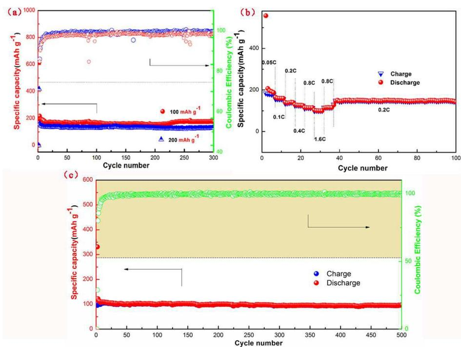
Fig. 6 (a) Cycle performances at current density 100 mA g<sup>-1</sup> and 200 mA g<sup>-1</sup> of the RGO/NPC electrode. (b) Rate performance of the RGO/NPC anode electrode. (c) Long cycle performance at 1000 mA g<sup>-1</sup> of the RGO/NPC anode electrode.
