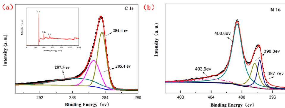
Fig. 4 (a) the XPS C 1s spectra of RGO/NPC, the inset picture is the XPS spectrum of RGO/NPC. (b) The XPS N 1s spectra of the RGO/NPC.
