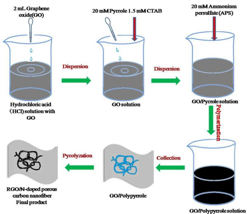
Fig. 1 Schematic of the RGO/NPC fabricate procedure.
