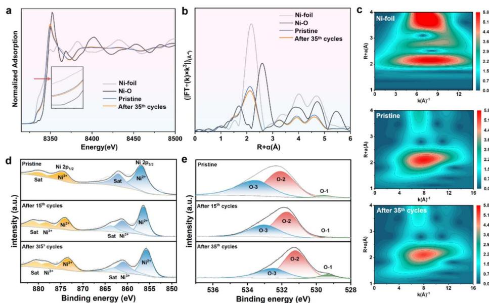
Fig. 5 (a) Ni K-edge XANES spectra, (b) the corresponding Fourier transforms of EXAFS spectra of Ni-BPM/NF-24 h and reference samples and (c) WT images. (d) Ni 2p XPS spectra and (e) O 1s XPS spectra of Ni-BPM/NF-24 h and after the 15th and 30th cycles, respectively. The peak corresponding to C=C from the C 1s high-resolution spectrum was at 284.8 eV and was used for charge calibration.<sup>41</sup>
