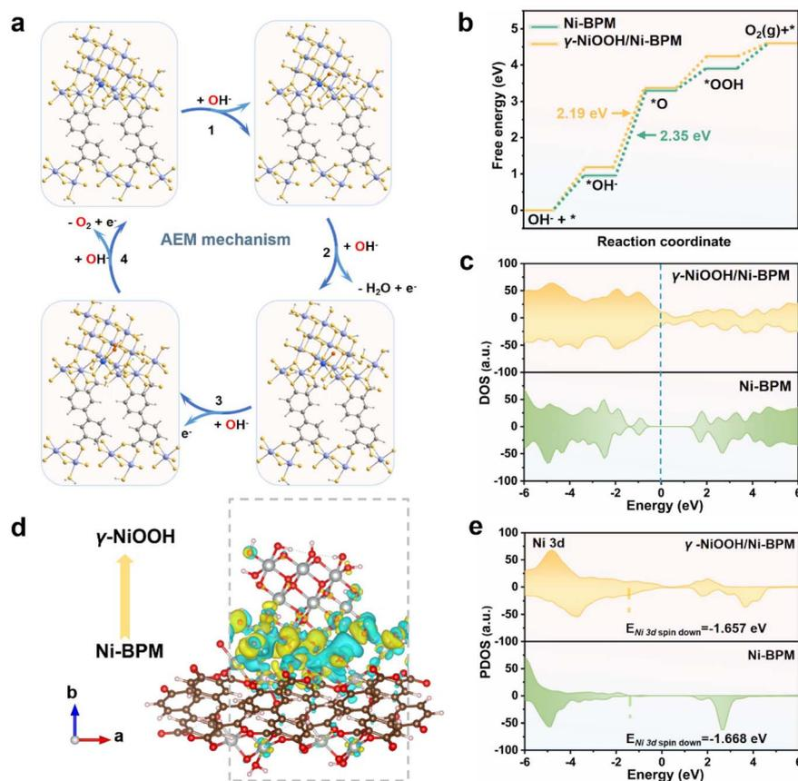
Fig. 4 (a) Illustration of intermediates formation during the OER based on the AEM mechanism; (b) free energy diagram of intermediate formation on Ni sites of Ni-BPM and  $\gamma\text{-NiOOH}/\text{Ni-BPM}$ ; (c) DOS plots of  $\gamma\text{-NiOOH}/\text{Ni-BPM}$  and Ni-BPM. (d) Distribution of interfacial charge. Yellow and blue represent the electron accumulation and dissipation areas, respectively. (e) PDOS plots of Ni 3d of  $\gamma\text{-NiOOH}/\text{Ni-BPM}$  and Ni-BPM.
