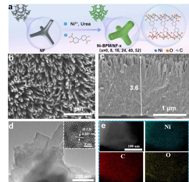
Fig. 1 (a) Schematic illustration of Ni-BPM/NF- $x$  ( $x = 8, 16, 24, 40$ , and  $52 \text{ h}$ ) electrode preparation. SEM (b and c), TEM and HRTEM (d) and TEM-EDX-mapping (e) images of Ni-BPM/NF-24 h.
