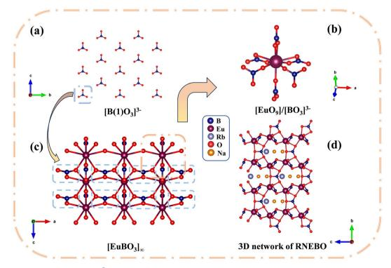
Fig. 1 (a) Coplanar arrangement of  $[B(1)O_3]^{3-}$  units between the  $[EuBO_3]_{\infty}$  layers. (b) Coordination of the  $[EuO_9]$  polyhedron with  $[BO_3]^{3-}$  units. (c)  $[EuBO_3]_{\infty}$  chains with  $[BO_3]^{3-}$  groups bridged between infinite chains along the b axis. (d) 3D network of RNEBO viewed along the a axis.
