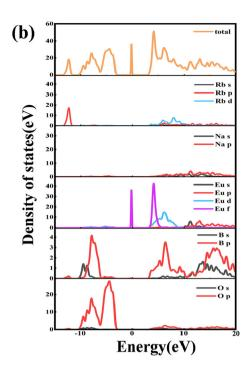
Fig. 6 (a) The electronic band structure calculated for RNEBO. (b) DOS and partial DOS projected for RNEBO.
