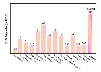
Fig. 4 Comparison of the SHG intensity with that of different crystals containing borates.31
