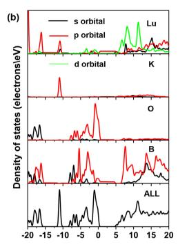
Fig. 4 (a) Band structure for the KLBO crystal. (b) PDOS and TDOS for the KLBO crystal.
