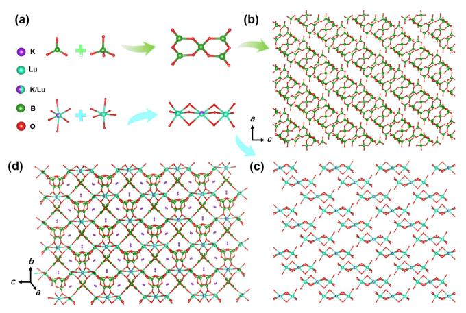
Fig. 2 Structure of KLBO. (a)  $[BO_3]$ ,  $[BO_4]$  units,  $[B_5O_{10}]$  groups and  $[K_{0.5}Lu_{2.5}O_{12}]$  functional building fragments. (b and c) Presentation of the  $[B_5O_{10}]$  and  $[K_{0.5}Lu_{2.5}O_{12}]$  groups, respectively. (d) 3D structural network.
