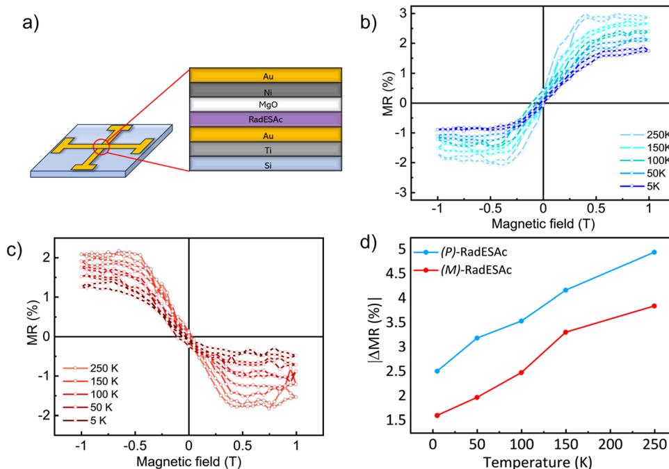
Fig. 4 (a) Scheme of the magnetoresistance device with magnification on the cross junction. Magnetoresistance percentage in the range  $\pm 1$  T of (b) **(P)-RadESAc@Au** and of (c) **(M)-RadESAc@Au** monolayers. (d)  $|\Delta\text{MR} (\%)|$  values as a function of the temperature for both the enantiomers.
