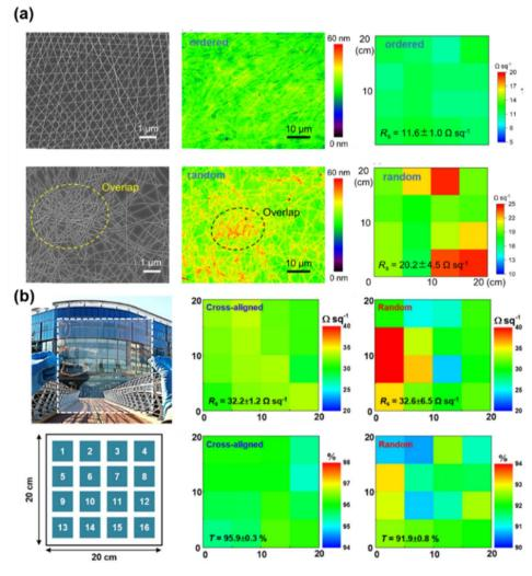
Fig. 5 Comparison of ordered and random Ag NW FTEs. (a) SEM images, AFM height profile, sheet resistance distribution. Reproduced with permission. Copyright 2024, Wiley-VCH. (b) Photograph of large scale (20 × 20 cm²) FTE and the mapping showing the distribution of sheet resistance and transmittance for the cross-aligned and random Ag NW FTEs. Reproduced with permission. Copyright 2017, American Chemical Society.
