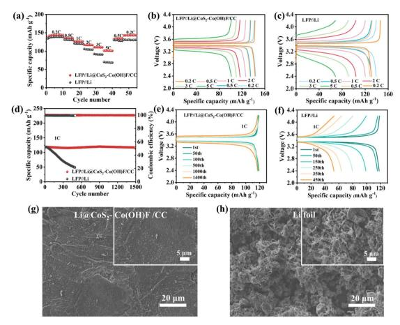
Fig. 7 (a) Rate capability and (b and c) charge-discharge profiles of LFP//Li@Li@CoS<sub>2</sub>-Co(OH)F/CC and LFP//Li full cells at various rates ranging from 0.2C to 5C. (d) Cycle performance and (e and f) charge-discharge profiles of LFP//Li@CoS2-Co(OH)F/CC and LFP//Li full cells at 1C. The SEM images of the corresponding anode for (g) LFP//Li@CoS2-Co(OH)F/CC and (h) LFP//Li full cells after 200 cycles at 1C.
