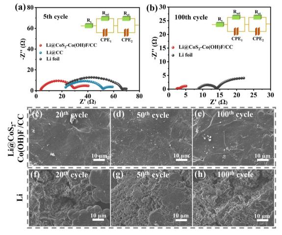
Fig. 6 (a and b) Nyquist plot of Li foil, Li@CC and Li@COS₂-Co(OH)F/CC-based symmetric cells at different cycles. SEM images of (c-e) the Li@CoS2-Co(OH)F/CC and (f-h) Li foil electrode after different cycles.
