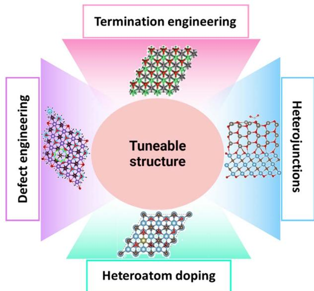
Fig. 8 Graphic illustration for different strategies for tuning MXene-based TMOs to enhance electrocatalytic performance, including termination engineering, defect engineering, heteroatom doping, and heterojunction formation.
