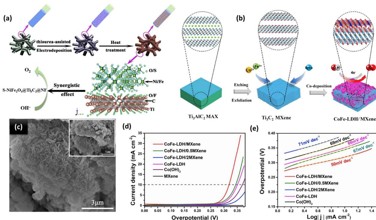
Fig. 11 (a) Schematic illustration of the fabrication of the S-NiFe<sub>2</sub>O<sub>4</sub>@Ti<sub>3</sub>C<sub>2</sub>@NF hierarchical network structure. Reproduced with permission from ref. 120. Copyright 2019, Elsevier. (b) Diagram illustrating the method for creating CoFe-LDH/MXene hybrids, (c) SEM image of CoFe-LDH/MXene nanohybrids, (d) LSV curves of samples, and (e) Tafel plots of samples. Reproduced with permission from ref. 121. Copyright 2019, Elsevier.
