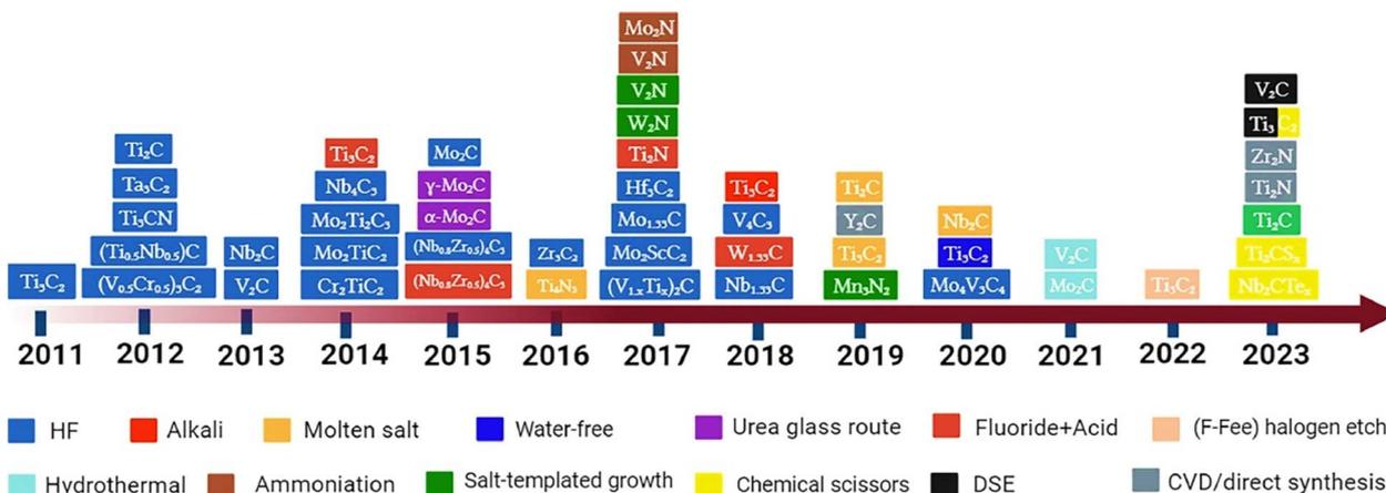
Fig. 4 Overview of various kinds of MXenes, their methods of production, and the corresponding timeframes. Reproduced with permission from ref. 45. Copyright 2023, Elsevier.
