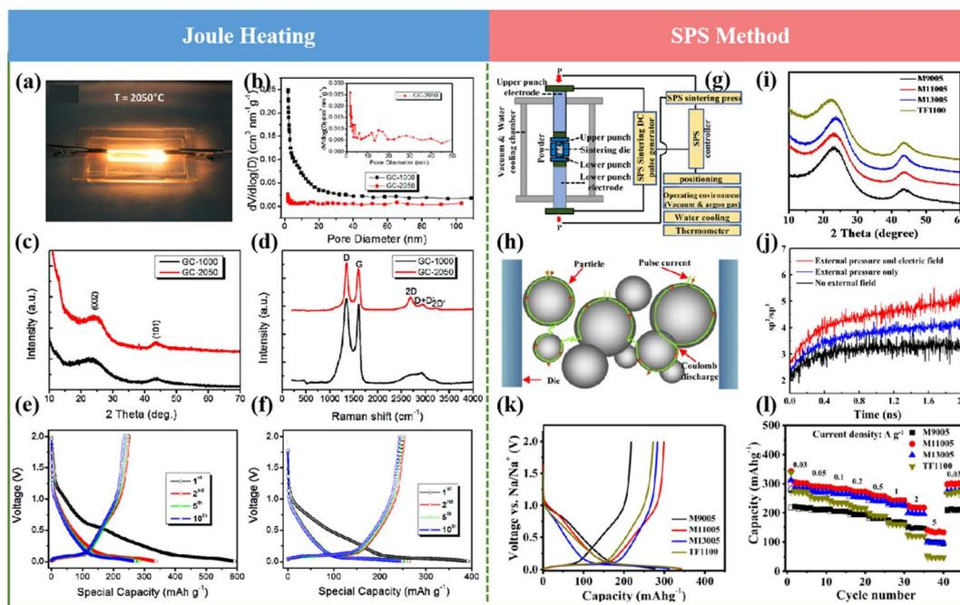
Fig. 9 (a) Photograph of switchgrass-derived HC *via* Joule heating. (b–d) Pore size distribution curves, XRD patterns, and Raman spectra of GC-2050 and GC1000. (e and f) Charge–discharge curves of GC-2050 and GC1000, (g) diagram of the SPS system, (h) annealing mechanism, (i) XRD patterns of HCs, (j) change in the structural composition of the materials and (k and l) electrochemical behaviors of HCs.
