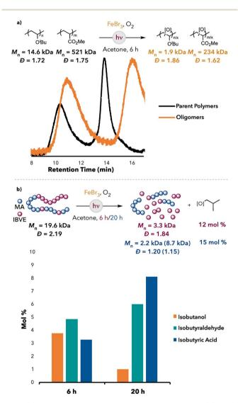
Fig. 5 (a) PIBVE and PMA mixture degradation with FeBr<sub>3</sub>. (b) Poly(-IBVE-co-MA) degradation results: Lower  $M_n$  peak (higher  $M_n$  peak).
