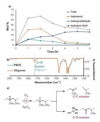
Fig. 2 (a) Kinetic study of PIBVE degradation under  $FeCl_3$  in (1:1) acetone/benzene co-solvent system. (b) IR spectrum of PIBVE and partially degraded oligomer. (c) Degradation study of poly(tert-butyl vinyl ether).
