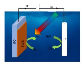
Fig. 17 Schematic mechanism of photoelectrochemical water splitting of  ${\rm Sb_2S_3\text{-}based}$  photocathode.
