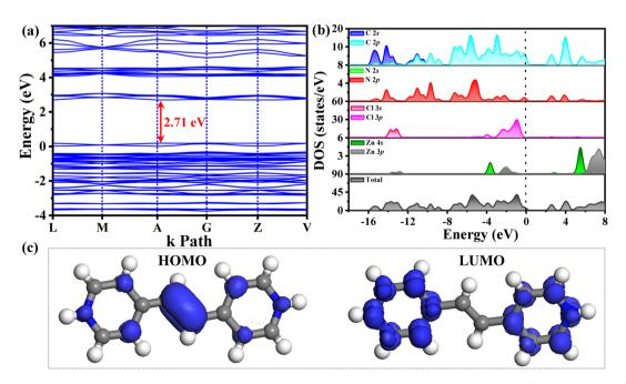
Fig. 4 Band structures and density of states of [DPE]ZnCl<sub>4</sub> (a and b); The frontier molecular orbits (HOMO and LUMO) of [DPE]ZnCl<sub>4</sub> (c).
