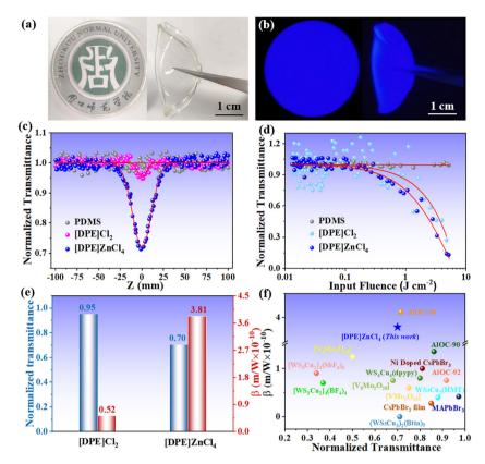
Fig. 3 (a and b) Photos of [DPE]ZnCl<sub>4</sub>@PDMS films in sunlight and ultraviolet light of 365 nm; (c) the open-aperture Z-scan diagrams of [DPE]Cl<sub>2</sub> and [DPE]ZnCl<sub>4</sub> at 532 nm; (d) the curves of normalized transmittance versus input fluence; (e and f) comparison of the minimum normalized transmittance and the nonlinear absorption coefficients for [DPE]Cl<sub>2</sub>, [DPE]ZnCl<sub>4</sub> and some representative crystalline materials reported.
