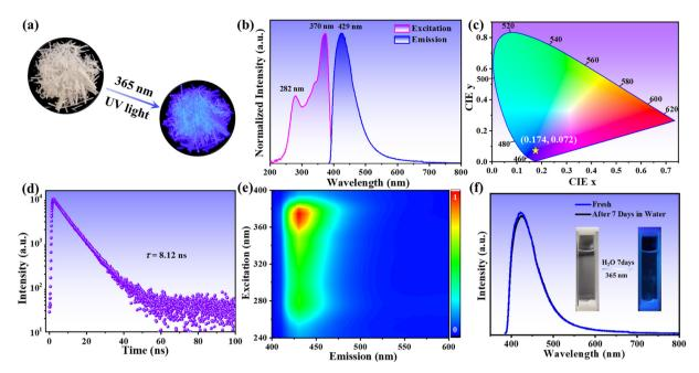
Fig. 2 Photoluminescence characterizations of [DPE]ZnCl<sub>4</sub>. (a) Photos of crystals in sunlight and ultraviolet light of 365 nm; (b) excitation and emission spectra; (c) the CIE coordinates; (d) the PL decay curve at 429 nm at 300K; (e) the 3D excitation and emission correlation map; (f) comparison of the PL spectrum before and after immersion in water for 7 days.
