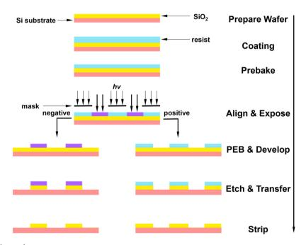
Fig. 2 The typical photolithography process.
