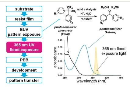
Fig. 8 Typical workflow of PSCAR and the generation of photosensitizers during EUV exposure, which could selectively sensitize the liberation of photoacids in the subsequent 365 nm flood exposure.
