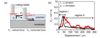
Fig. 4 (a) Schematic representation of SAICAS measurement, showing cutting modes and detecting forces along the directions vertical and horizontal to the interface. (b) Horizontal force ( $F_h$ ) profile for the PMMA L & S film before and after annealing, measured in the direction perpendicular to the line pattern.
