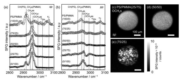
Fig. 5 SFG spectra for PS/PMMA blend films with different bulk compositions with (a) sp and (b) pp polarization combinations. SFG images for PS/PMMA (c) (25/75), (d) (50/50), and (e) (75/25), respectively. All blend films were annealed at 433 K for 48 h under vacuum.
