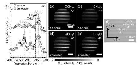
Fig. 2 (a) SFG spectra in the CH region with the sp polarization combination for a thin PMMA L&S film before (top) and after (bottom) annealing at 433 K for 24 h. SFG images for OCH<sub>3s</sub> and CH<sub>2as</sub> signals with the sp polarization combination for the (b and c) as-spun and (d and e) annealed films. (f) A digital microscopic image of the film. The angle formed with the line pattern ( $\omega$ ) is shown.
