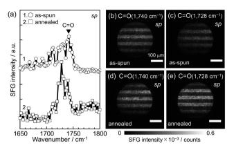
Fig. 3 (a) SFG spectra in the C $\equiv$ O region with the sp polarization combination for the thin PMMA L&S film before (top) and after (bottom) annealing at 433 K for 24 h. (b–e) SFG images for C $\equiv$ O signals with the sp polarization combination obtained at IR wavenumber of (b and d) 1740 cm $^{-1}$  and (c and e) 1728 cm $^{-1}$  for the as-spun and annealed films, respectively.
