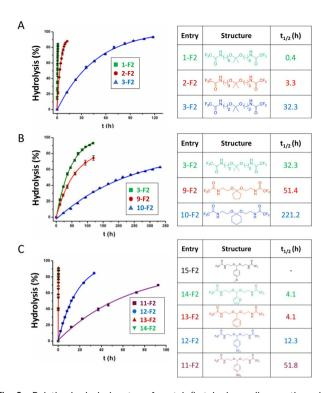
Fig. 2 Relative hydrolysis rates of acetals/ketals depending on the substituents at the R<sub>1</sub>, R<sub>2</sub> and R<sub>3</sub> positions, with varying the (A) distance between the electron-withdrawing amide moiety and ketal moiety, (B) substituents effects of acrylic and cyclic ketones, (C) effects of electronwithdrawing and electron-donating substituents. The solid lines are fitting curves.<sup>27</sup> (Copyright 2017 American Chemical Society).
