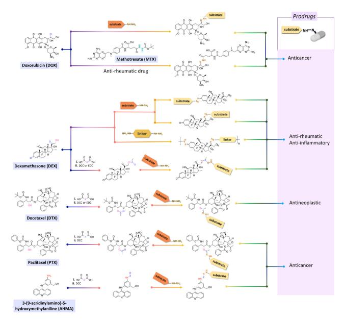
Fig. 15 Chemical structure and scheme for modifying active agents bearing ketone groups to produce hydrazone derivatives. Anticancer agents (doxorubicin, methotrexate, paclitaxel and 3-(9-acridinylamino)-5-hydroxymethylaniline), anti-rheumatic and anti-inflammatory agents (dexamethasone), or antineoplastic agents (docetaxel) can be directly reacted with substrates containing hydrazine groups or *via* aldehyde-based spacers.
