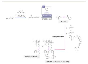
Fig. 25 Scheme of the synthesis of 2-(1-(benzoyloxy)-ethyoxyl)ethyl methacrylate (BEEMA) and its copolymerization with either methyl methacrylate or 2-((4-((((2-(1H-indol-3-yl)ethyl)carbamoyl)oxy)-methyl) phenyl)disulfanyl)ethylmethacrylate (IDEMA) and methyl methacrylate.  $^{179}$
