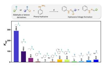
Fig. 14 Relative formation rates ( $K_{rel}$ ) of hydrazones from a selected set of aldehydes and ketones at pH 7.127 The relative reaction rates refer to the hydrazone formation between either aldehyde or ketones and phenylhydrazine [ $K_{rel}(4-methoxybenzaldehyde) = 1$ ]. 67
