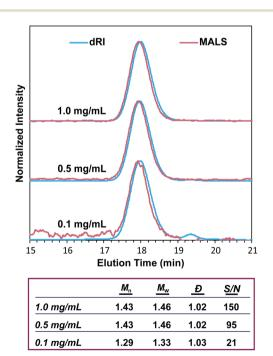
Fig. 7 SEC-MALS chromatograms of a 1.3 kg  $\mathrm{mol}^{-1}$  PS standard at various concentrations, showing the ability for SEC-MALS to accurately characterize this oligomer even at low concentrations. S/N denotes signal-to-noise ratio.
