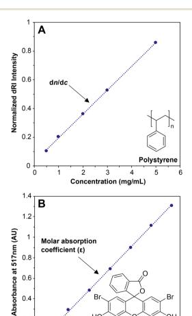
Fig. 1 (A) Offline dn/dc experiment using various concentrations of a nominal 30 kg mol<sup>-1</sup> polystyrene (PS) standard in THF, where the slope is equal to the dn/dc: (B) UV-vis experiment using various concentrations of eosin Y in water, where the slope is equal to the molar absorption coefficient ( $\varepsilon$ ).
