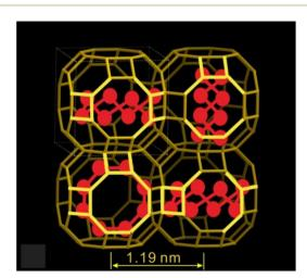
Fig. 1 Schematic view of the LTA framework with Te<sub>8</sub> rings in large
