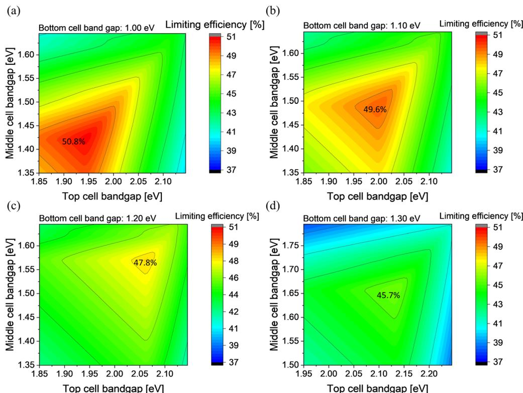
**Fig. 3** Theoretical efficiencies in the radiative limit for triple-junction solar cells for a bottom cell absorber with a bandgap of (a) 1.00 eV, (b) 1.10 eV, (c) 1.20 eV, and (d) 1.30 eV. The optimum top and middle cell bandgaps in each case are (a) 1.94 eV and 1.42 eV, (b) 2.00 eV and 1.49 eV, (c) 2.06 eV and 1.57 eV, and (d) 2.13 eV and 1.66 eV.
