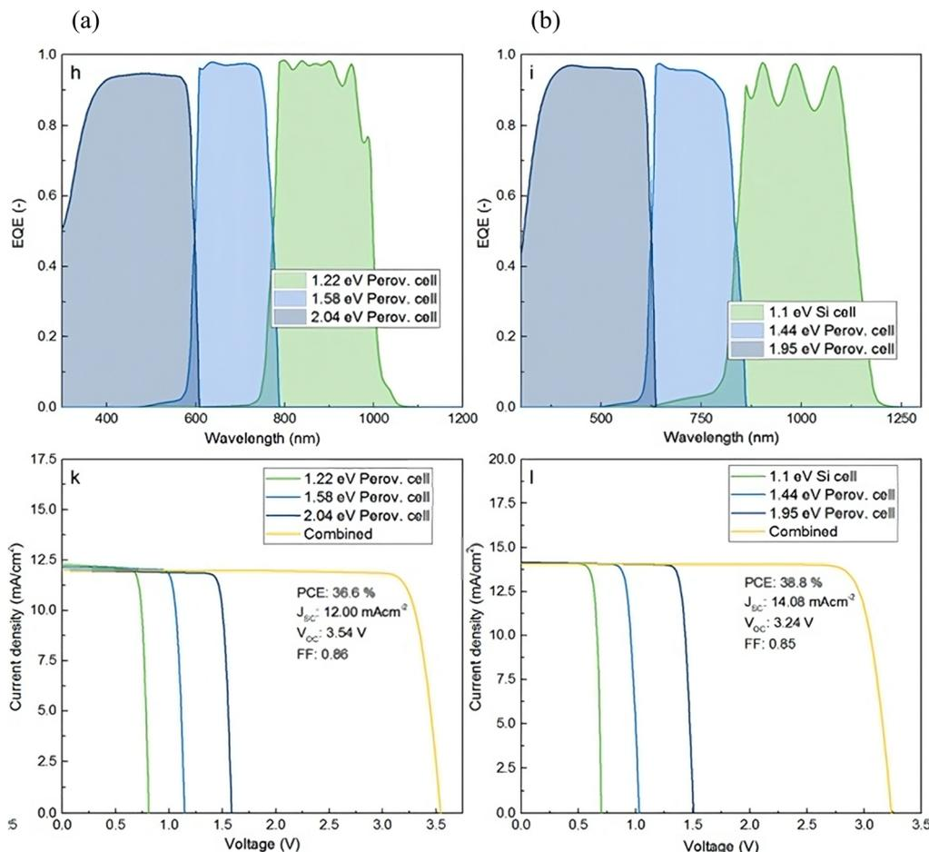
Fig. 4 Simulated external quantum efficiency (EQE) and current density–voltage ( $jV$ ) curves for maximum practical PCE (a) 36.6% for an all-perovskite triple-junction solar cell with perovskite's bandgaps of 1.22 eV, 1.58 eV, and 2.04 eV for the subcells and (b) 38.8% for a perovskite/perovskite/silicon triple-junction solar cell with bandgaps of 1.44 eV and 1.95 eV for perovskite subcells. Reproduced with permission from ref. 27, Copyright © 2017, American Chemical Society.
