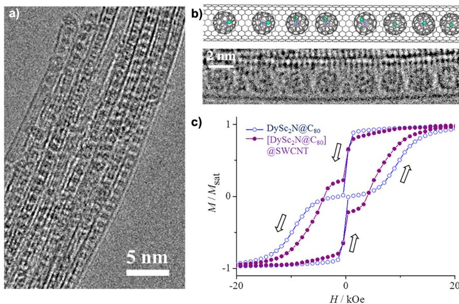
Fig. 11 (a) and (b) TEM images and structural model of  $[\text{DySc}_2\text{N@C}_{80}]@\text{SWCNT}$ . (c) Magnetic hysteresis loops for  $\text{DySc}_2\text{N@C}_{80}$  (open circles) and  $[\text{DySc}_2\text{N@C}_{80}]@\text{SWCNT}$  (filled circles) at 1.8 K. Arrows indicate the direction of the measurements. Reproduced with permission from ref. 236 (Copyright 2018, American Chemical Society).
