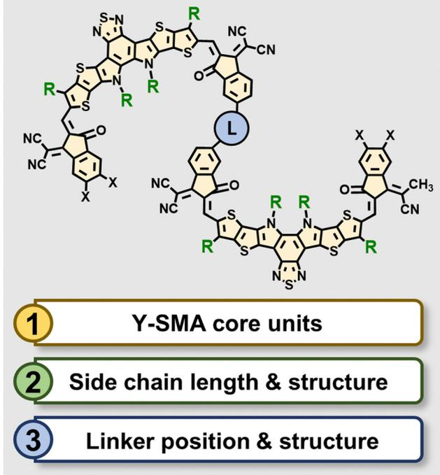
Fig. 8 General design considerations for Y-based DSMA.
