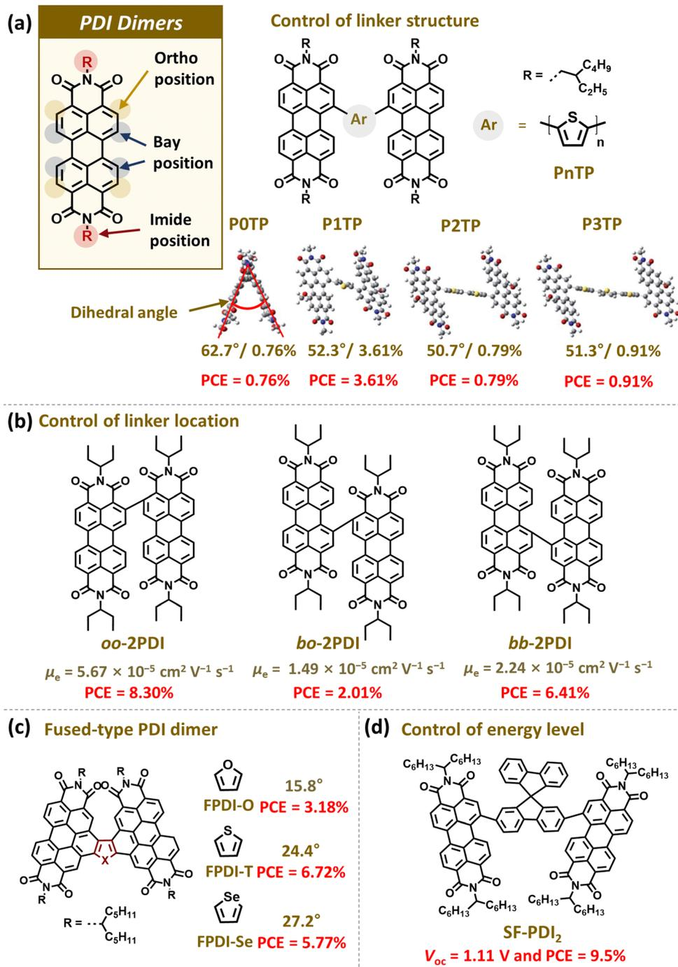
Fig. 5 Representative examples of PDI-based dimer acceptors; (a) P0TP, P1TP, P2TP, and P3TP, (b) oo-2PDI, bo-2PDI, and bb-2PDI, (c) FPDI-O, FPDI-T, and FPDI-Se, and (d) SF-PDI<sub>2</sub>. Reproduced from ref. 121 with permission from the Royal Society of Chemistry, copyright 2024.
