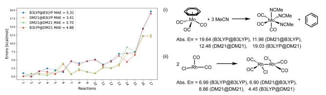
Fig. 4 (left) Errors of the four method combinations for MOR17 dataset. def2-TZVP basis set was used and the D3(BJ) correction has been added to all results. (right) Example of reactions in MOR17 with large errors.
