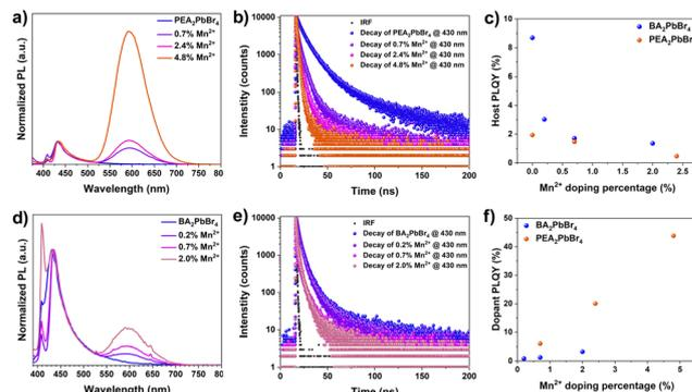
Fig. 3 (a) PL spectra of  $\text{Mn}^{2+}:\text{PEA}_2\text{PbBr}_4$ . (b) TRPL of  $\text{Mn}^{2+}:\text{PEA}_2\text{PbBr}_4$ . (c) Host PLQY against  $\text{Mn}^{2+}$  percentage. (d) PL spectra of  $\text{Mn}^{2+}:\text{BA}_2\text{PbBr}_4$ . (e) TRPL of  $\text{Mn}^{2+}:\text{BA}_2\text{PbBr}_4$ . (f) Dopant PLQY against  $\text{Mn}^{2+}$  percentage.
