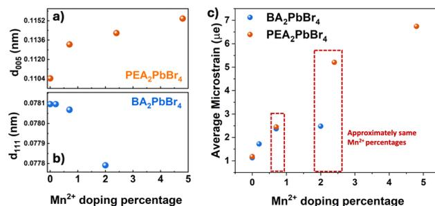
**Fig. 2** The change in  $d$ -spacing against  $\text{Mn}^{2+}$  concentration of (a) the (005) plane in  $\text{PEA}_2\text{PbBr}_4$  (b) the (111) plane in  $\text{BA}_2\text{PbBr}_4$  and (c) microstrain vs.  $\text{Mn}^{2+}$  doping percentage.
