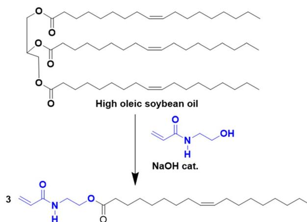
Fig. 4 Synthesis of HOSBM by transesterification reaction.
