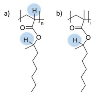
**Fig. 6** Abstractable hydrogen atoms of (a) 2-octyl acrylate and (b) 2-octyl methacrylate biobased homopolymers.
