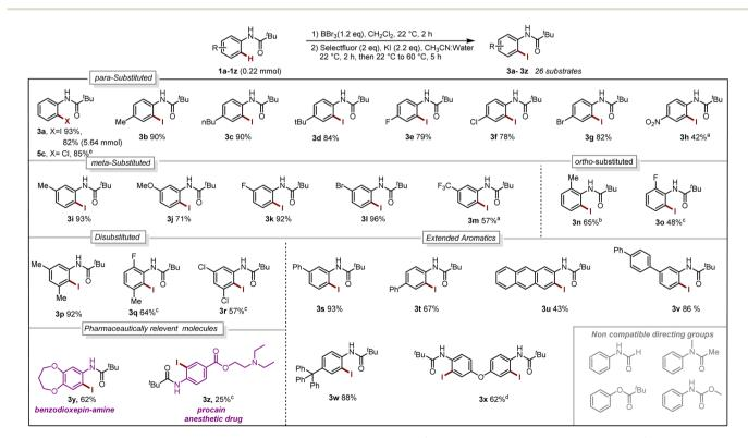
Scheme 1 Reaction Scope. Iodination (1a-1z 0.22 mmol): 2.2 mmol of BBr<sub>3</sub>, bstep-1 for 16 h. cStep-1 at 40 °C, 16 h. d0.48 mmol of BBr<sub>3</sub>, 0.88 mmol of Selectfluor, 0.92 mmol of KI. Chlorination: 0.1 mmol of 4a, 0.1 mmol of chloramine T trihydrate, CH<sub>3</sub>CN:Water, 70 °C, 4 h (for reaction condition see Section 4.4 in ESI†).
