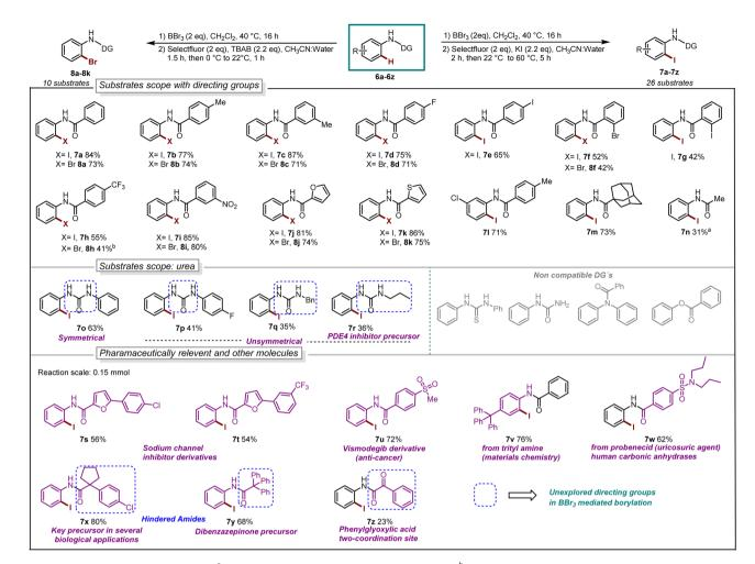
Scheme 2 Reaction scope, iodination: aBBr<sub>3</sub> (0.66 mmol), 60 °C, 24 h. Bromination: step-2 at 40 °C, 1.5 h.
