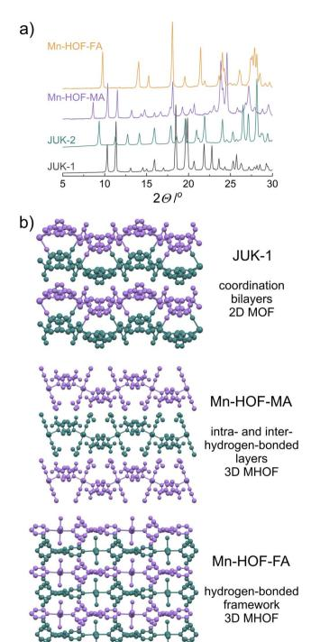
Fig. 2 Structural transformation between JUK-1 and Mn-HOFs. (a) PXRD patterns for JUK-1 and Mn-HOFs, compared with related JUK-2. (b) Stacked coordination bilayers in the initial JUK-1 (top), and the resulting: stacked hydrogen-bonded layers in Mn-HOF-MA (middle) and 3D hydrogen-bonded network in Mn-HOF-FA (bottom), all packing views along the *c* axes. The layers in JUK-1 and Mn-HOF-MA are stabilized by interlayer hydrogen bonds.
