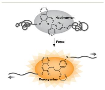
Fig. 1 Mechanophores covalently incorporated into polymer chains undergo productive chemical reactions in response to mechanical force. The mechanochromic transformation of naphthopyran is illustrated
