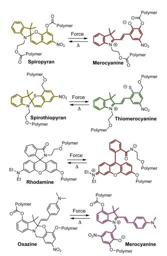
Scheme 3 Examples of mechanochromic mechanophores that undergo ring-opening reactions upon mechanochemical activation to produce thermally reversible colored dyes.
