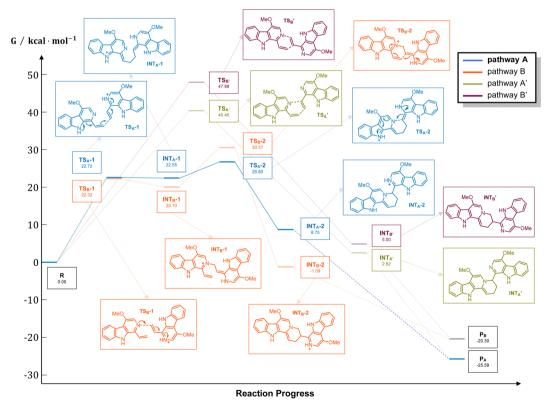
Scheme 3 Energy profile of the aza-[4 + 2] cycloaddition. For pathways A and B,  $R = 1 \times$  dehydrocrenatine (10a) and  $1 \times$  protonated dehydrocrenatine; for pathways A' and B',  $R = 2 \times$  dehydrocrenatine.  $P_A =$  picrasidine G (1),  $P_B =$  isopicrasidine G. Calculation at WB97XD/6-311++G(2d,p)//WB97XD/6-31G(d) at 403.15 K. Gibbs free energies ( $\Delta G$ ) are in kcal mol<sup>-1</sup>.
