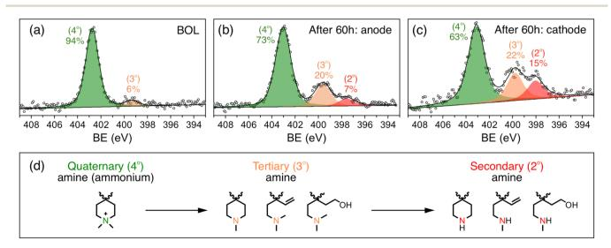
Fig. 4 N 1s XPS spectra of the catalyst layer at (a) the beginning of life (BOL) and the (b) anode and (c) cathode after 60 hours of stability testing. (d) Quaternary and possible tertiary and secondary amine structures corresponding to N 1s XPS peaks.
