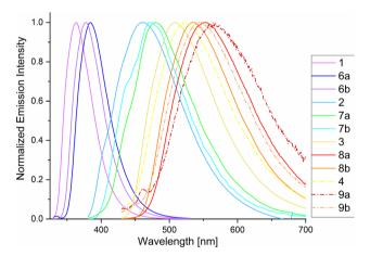
Fig. 5 Photoluminescence spectra of 1–4 and 6–9 a,b in MeCN at RT (for  $\lambda_{ex}$ , see Chapter 4, ESI†).
