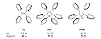
Fig. 1 Molecular structures of AIEgens tetraphenylethene (TPE),  $^{10}$  hexaphenylsilole (HPS),  $^{11}$  and pentaphenylphosphole oxide (PPPO) $^{12}$  and their fluorescence quantum yields in solution ( $\Phi_{\rm F}$ ) and the solid state ( $\Phi_{\rm F}$ (solid)).
