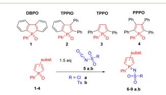
Scheme 2 Synthesis of sulfonylimino phospholes 6-9 a,b
