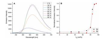
Fig. 6 Photoluminescence spectra of **9b** in different MeCN/water mixtures ( $\lambda_{\rm ex}=398$  nm) (A) and emission intensity of **8b** and **9b** in MeCN/water for increasing water content ( $f_{\rm w}$ ) (B).
