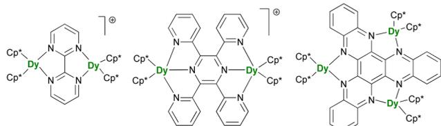
Fig. 9 Molecular structures of  $\{[(\text{Cp}^*)_2\text{Dy}]_2(\mu\text{-bipym})\}^+$ ,<sup>196</sup>  $\{[(\text{Cp}^*)_2\text{Dy}]_2(\mu\text{-tppz})\}^+$ ,<sup>197</sup> and  $(\text{Cp}^*)_6\text{Dy}_3(\mu_3\text{-HAN})$ .<sup>198</sup>
