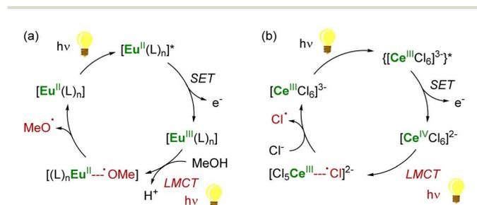
Scheme 7 LMCT-induced homolysis in  $\text{Eu}^{\text{III}}/\text{Eu}^{\text{II}}$  (a)<sup>146,149</sup> and  $\text{Ce}^{\text{IV}}/\text{Ce}^{\text{III}}$  (photo)catalysis (b).<sup>90</sup>
