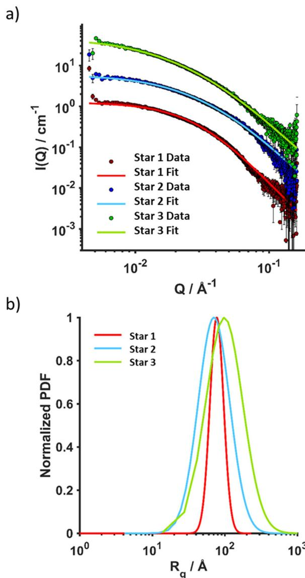
**Fig. 3** SAXS analysis in DMF ( $2 \text{ mg mL}^{-1}$ ,  $25^\circ\text{C}$ ) of Star 1, Star 2 and Star 3. (a) Overlay of raw data and fittings (polydisperse star polymer model), (b) radius of gyration fit to a lognormal distribution.
