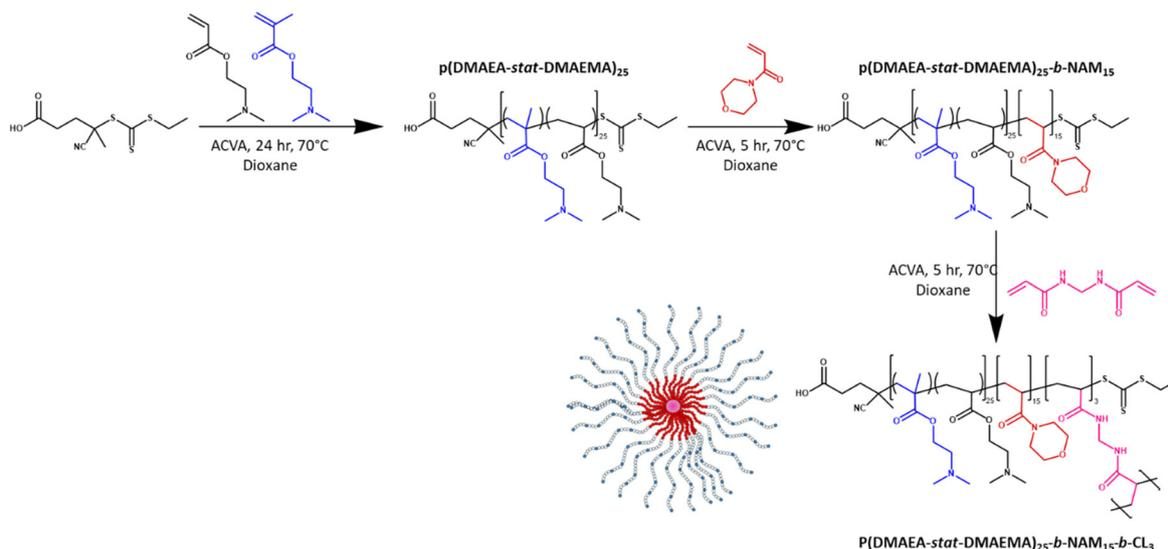
**Scheme 1** Synthesis of p(DMAEA-*stat*-DMAEMA)<sub>25</sub>-*b*-NAM<sub>15</sub>-*b*-CL<sub>3</sub> star copolymer by the arm-first approach.
