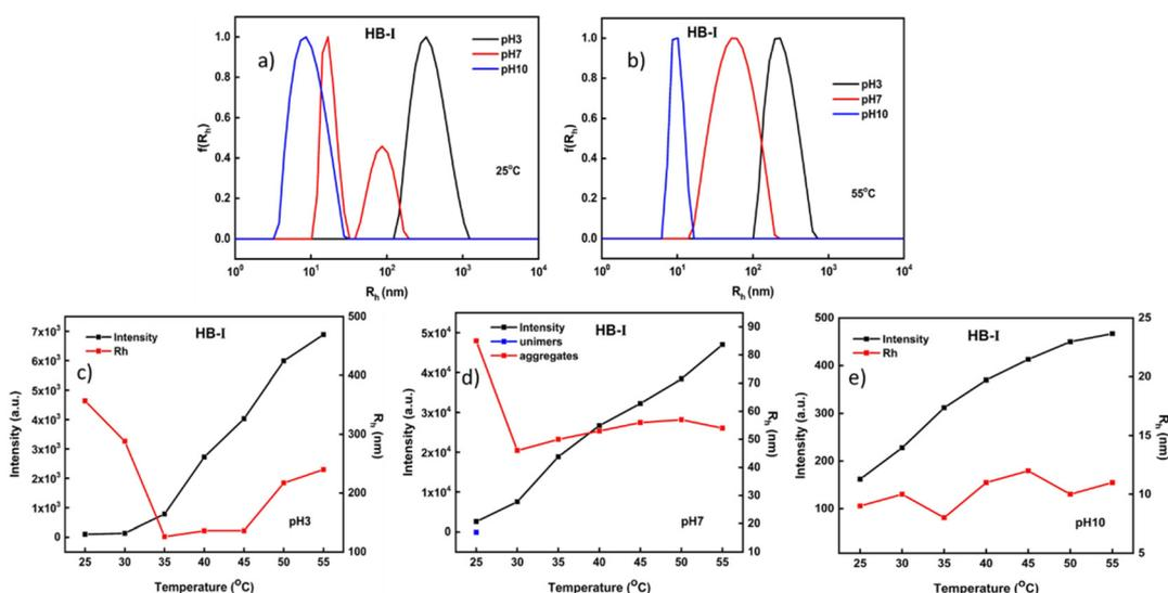
Fig. 4 Light scattering results for the HB-I hyperbranched copolymer solutions: size distributions from DLS (upper row: a and b) and variation of the scattered intensity and  $R_h$  as a function of pH and temperature (lower row: c, d and e).
