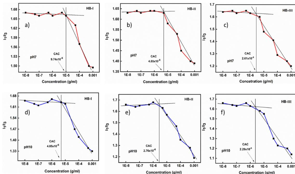
Fig. 3 CAC determination for P(DEGMA-co-DIPAEMA) hyperbranched copolymers at pH 7 (upper row: a, b and c) and pH 10 (lower row: d, e and f).
