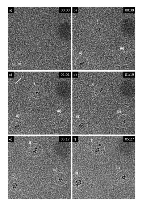
Fig. 2 Sequential images from an in situ LP-TEM movie showing (a)-(b) formation and (c)-(f) arrangement of primary particles when a dose rate of  $16.7 \times 10^6$  Gy s<sup>-1</sup> is applied. Primary CeO<sub>2</sub> particles can be resolved and evaluated quantitatively, because of lower thickness of the liquid in comparison to Fig. 1. (See also according video "V02\_LP-TEM\_CeO2-nanoparticles"; time given as mm:ss).
