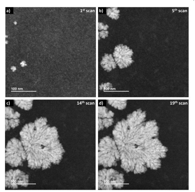
Fig. 5 Sequential in situ ADF imaging in LP-STEM. An average dose rate of  $5.9 \times 10^6$  Gy s<sup>-1</sup> is applied. (a) Already within the first scan, the aggregates become visible. (b) Continuous growth of aggregates while no formation of the additional ones is observed. (c) The appearance of the growing aggregates changes from isotropic to branched structures. (d) Further development of branched structures to larger sizes (video "V03\_LP-STEM\_CeO<sub>2</sub>-nanoparticles.avi").
