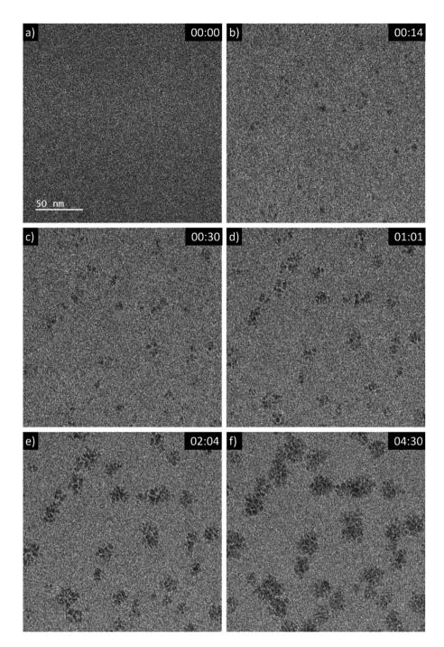
Fig. 1 Sequential images from an *in situ* LP-TEM movie showing the formation of aggregates (see video "V01\_LP-TEM\_CeO<sub>2</sub>-nanoparticles.avi", time given as mm:ss). A dose rate of  $16.7 \times 10^6$  Gy s<sup>-1</sup> is applied.
