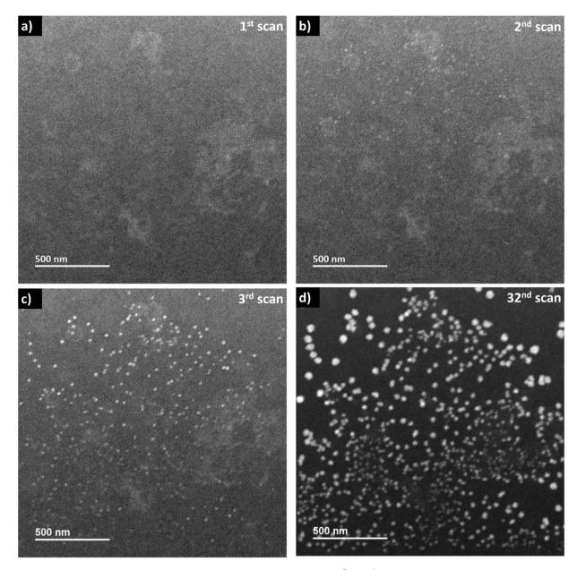
Fig. 6 Sequential in situ ADF imaging in LP-STEM. An averaged dose rate of 2.4 × 10<sup>5</sup> Gy s<sup>-1</sup> is applied. (a) Initial scan. (b) Nano-sized aggregates become visible in the second scan and (c) their contrast increases during exposure. (d) The projected size of the aggregates increases constantly while almost no new ones are formed. (see video "V04\_LP-STEM\_CeO2-nanoparticles.avi").
